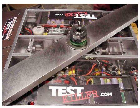
the bar through the friction forces caused by a large washer. This washer is pressed against the bar using a spring element (in green in the figure), held by the threaded collars. Note that two collars are used in this case, to improve strength and to act together as counter nuts. Note also that flat surfaces were machined on the collars to make it easier to get tightened, with an open-end wrench.
