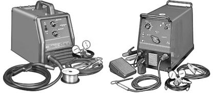
compromise strength. These equipments rely on an inert gas that is released during the welding process, shielding the heated part from the surrounding atmospheric gases, which would react to and weaken the weld.
