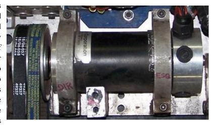
can be found at <a href="www.robotmarketplace.com">www.robotmarketplace.com</a>. This method, besides much more resistant, is as practical as using clamps, because to switch the motor it is enough to deal with only 4 screws.
